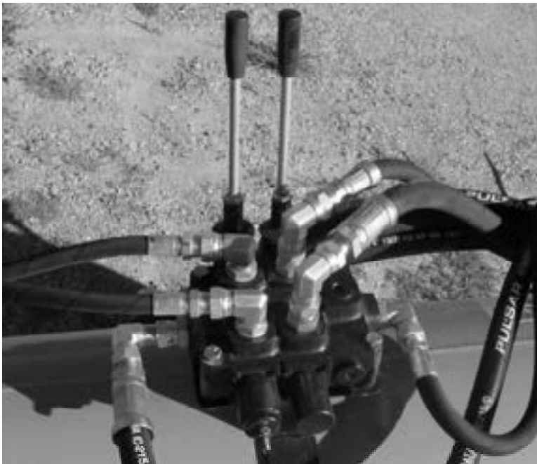
Figure 17. Power Swing Control Valve
